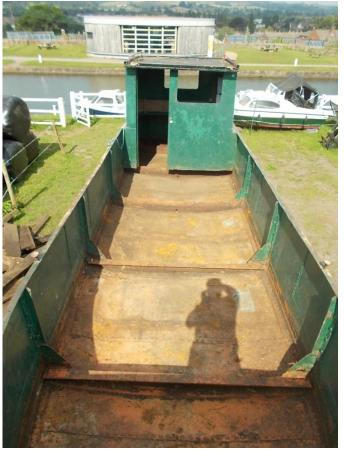
Philip Brind and a welding contractor he has worked with on several other canal boats in recent years have looked the boat over but feel that the cost of shot-blasting, re-plating and painting the floor of the boat is likely to be considerably greater than the cost of purchasing a new boat.
